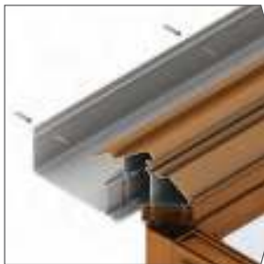
Fix box gutter to existing wall
