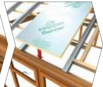
Install external insulation
